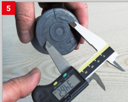
5 Transfer the diameter to a multilayer insert
