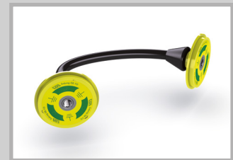
Flexible penetration grounding GE-FD/(L) Flexible, insulated duct to be encased flush in concrete; on both sides with connection M12. For wall thickness from 150 - 500 mm
