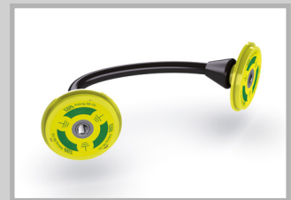
Flexible penetration earthing GE-FD/(L) Flexible, insulated entry to be encased flush in concrete; on both sides with connection M12. For wall thickness from 150 - 500 mm
