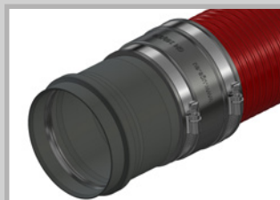
Pipe fitting SM110 or SM160 For connection of a smooth-walled pipe SM110: for pipe with outside diameter 110 mm; Available for KSS110 SM 160: for pipe with outside diameter 160 mm; Available for KSS150
