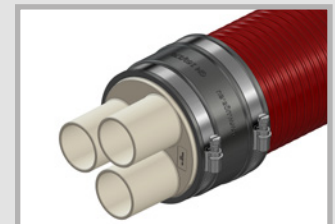
System cover D3 With three connection pieces for sealing up to three cables using shrink technology D3/59: Three connection pieces with \varnothing 59 mm for cables with \varnothing 22 – 57 mm; Available for KSS150 and KSS125 D3/46: Three connection pieces with \varnothing 46 mm for cables with \varnothing 16 – 44 mm; Available for KSS110 D3/30: Three connection pieces with \varnothing 30 mm for cables with \varnothing 7 – 28 mm; Available for KSS80
